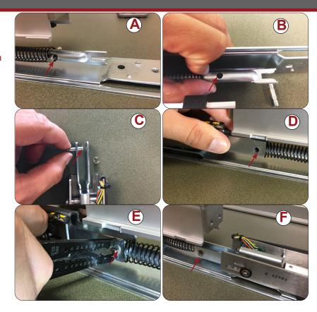
Once the kit is secure with the pin, lift up and insert back screw into the bottom dogging hole. Do not tighten until device is assembled.
