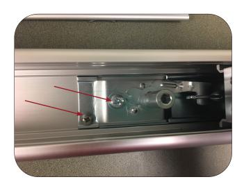
**4.** Once removed, slide push pad assembly out the back of the device.
