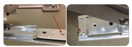
10. Once kit is connected, flip device over and put screws back in dogging holes.
